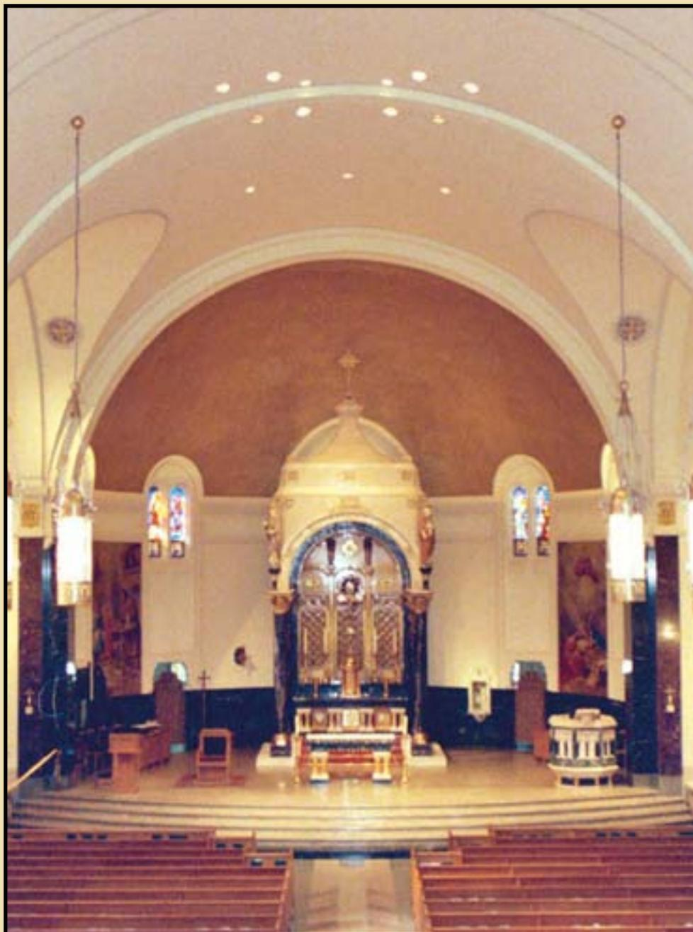
A new color scheme was introduced with a combination of decorative effects to highlight the architecture of this beautiful Church. Extensive scaffold was installed to decorate the ceiling area as well as the clerestory walls. Marble pilasters, lower side wall areas, mosaics and baldachino were cleaned, pointed and treated to a luster finish.
