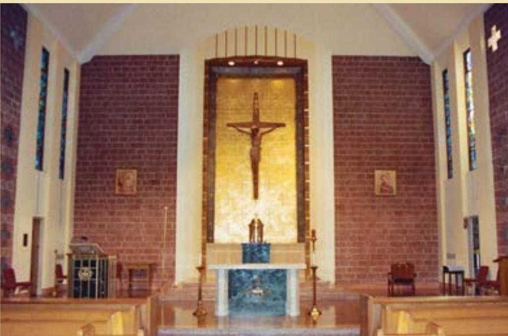
The redesigning of the sanctuary platform included the removal of the existing original Altar from the reredos wall, the continuation of the reredos wall to the floor with marble including moldings on both sides and the repair of the floor as required. The original Altar was modified in size and shape and constructed in a more forward position. A new top was supplied and overall fabrication included the reuse all green marble and columns.
